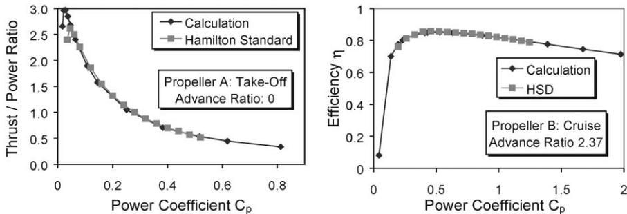
Fig. 6. Thrust/power ratio and efficiency.
