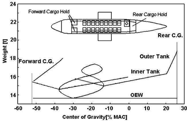
Fig. 9. Typical cabin layout and loading diagram.
