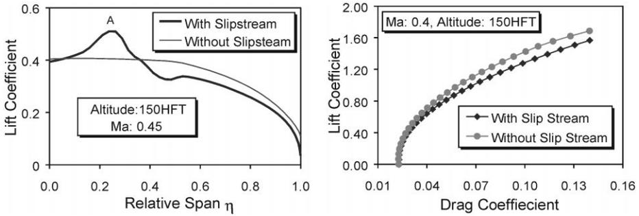
Fig. 8. Lift distribution and polar diagram.
