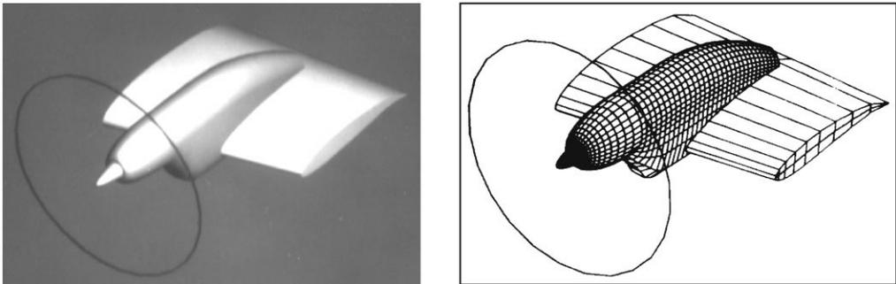
Fig. 10. Shaded- and hidden-line model.
