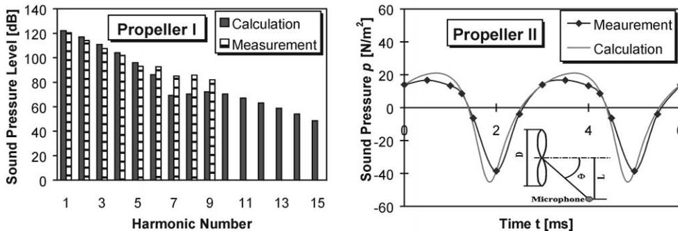
Fig. 7. Verification of acoustics analysis: propeller pressure signal and sound spectrum.
